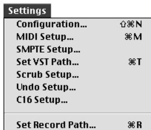
The Settings menu allows you to configure PARIS for optimal performance, MIDI operations, use of VST Plug-In Effects, and recording.
