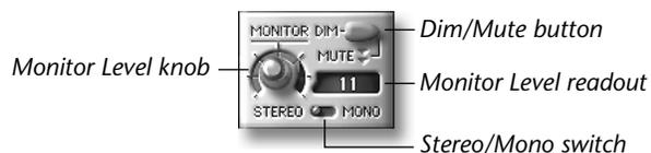
The Monitor controls set the listening environment of the entire current Project; therefore, these controls are available in each SubMix's Mixer. They allow you to set the listening volume, temporarily dim the volume without losing your original listening level, and audition your Project in mono.
