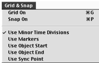
The Grid & Snap Menu provides options that control the on/off status of the Editor Window's alignment Grid, its Snap feature, the fineness of time measurements used by the Grid, and allows you to activate Marker, and Objects and sync point times for use by the Grid. The items in this menu duplicate the actions of the buttons on the Grid & Snap bar, as described below.
