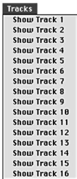
The options in this menu controls the number of Channel strips available in the Mixer Window. To select the desired number of Channel strips, click the menu and drag to select the desired item—a checkmark will appear next to it.
