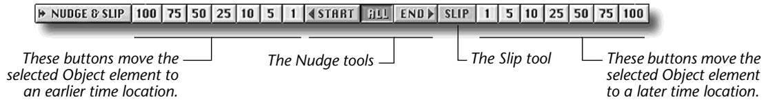
Each Nudge or Slip tool becomes activated when its button is clicked—these tools determine the Object element that will be moved. The numbered buttons to the left and right of the Nudge and Slip tools move the selected component of the Object earlier or later in time, respectively, by 1-millisecond, 5-millisecond, 10-millisecond, 25-millisecond, 50-millisecond, 75-millisecond or 100-millisecond intervals. You can click the buttons in any order achieve the desired result.
