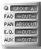
The controls of several channels can be grouped so that moving a control on one channel will move the same control on another. Faders, Pan controls, EQ controls and the Aux Controls can be grouped.
