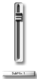
Click and drag the SubMix Master Fader to reduce the overall volume of the SubMix. The current amount of reduction to the SubMix's volume is shown in the SubMix Master Fader readout. When working with a collapsed SubMix Master Fader module, click and drag directly on the SubMix Master Fader readout.
