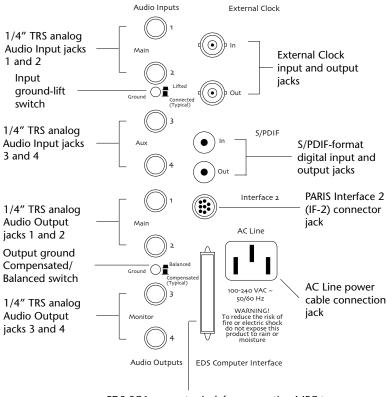
EDS-SC6 connector jack for connecting MEC to EDS-1000 PCI card
