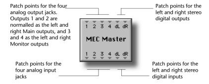
You can set the levels for each pair of analog inputs and outputs in the Patch Bay Window's Master Module Configuration dialog. Inputs 1 and 2 are labeled in the dialog as "Main In Level," Inputs 3 and 4 are "Aux In Level," Outputs 1 and 2 are "Main Out Level," and Outputs 3 and 4 are "Control Room Out Level." These names reflect the default—or "normalled"— connections for the Master Module's inputs and outputs.
